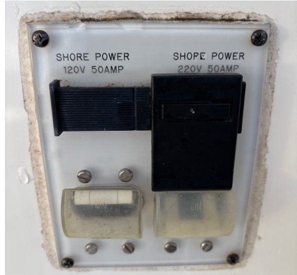
Breaker for each connection. Note that 50 amp/125v is ON (which is typical)
