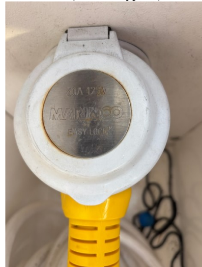
Middle plug – Use with 50amp to 30 amp adapter, when 30 amp 125V power is available at the dock.
