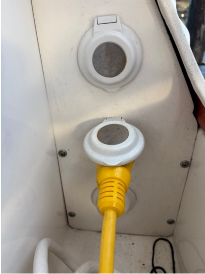
Available shore power connections, located in aft storage locker. Bottom is cable TV and phone.
