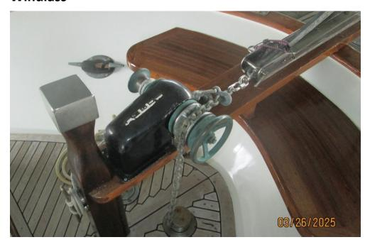
The WINDLASS POWER SWITCH is located at the lower helm just below helm. The primary WORKING ANCHOR is CRQ and is attached to 300 ft chain and passed through the deck from the ANCHOR LOCKER.
