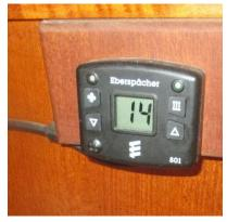
Set the THERMOSTAT to the desired temperature by pressing and holding the up or down arrows until the desired temperature is displayed. Quickly depressing the up or down buttons will display what the furnace is set for. When you release the up or down arrow the current cabin temperature is indicated.
