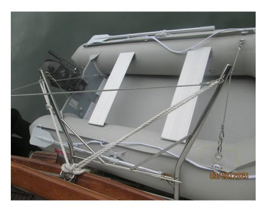
Your Saturn Inflatable DINGHY with a 6 hp four stoke engine is stored on the rear davit system at the stern of the boat. It has a capacity of about 1000 pounds (motor, equipment, and 4 people). A throwable cushion with survival kit, whistle, patch kit, and engine shut off clip, as well as life vests are found under the salon bench seat. Place the needed number of life vests and the throw cushion in the boat.
