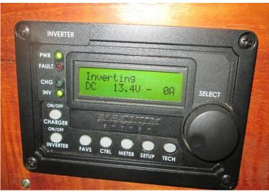
The INVERTER provides AC power to the 110-volt receptacle plugs (i.e., the microwave oven) when the boat is disconnected from shore power. The inverter does not provide power to the water heater or the battery charger. Your inverter panel is located left of the ship's wheel with a push button on/off. switch. Make certain that it is on. The actual inverter is located on the aft bulkhead of the engine room.
