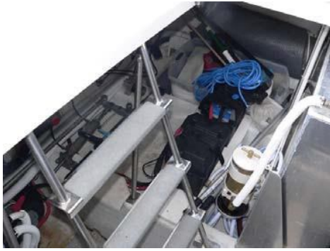
A look into the lazarette; the ladder eases engine room access.
