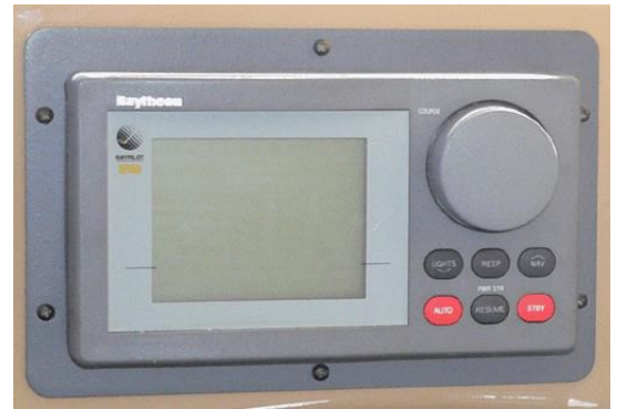
(above) Autopilot control at lower helm. (below) Flybridge unit.
