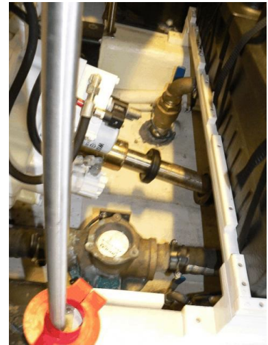
Port main engine sea strainer in foreground; its valve is just on the far side of shaft, with blue handle on far side “up”/open.
