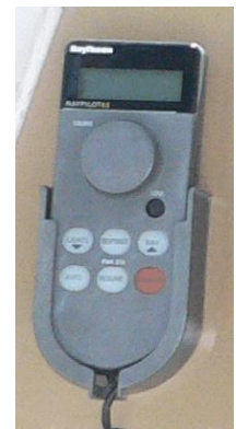
(above) Autopilot control at lower helm. (below) Flybridge unit.
