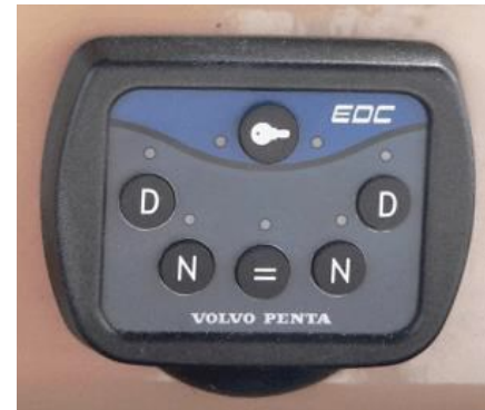
The electronic controls for the engines have six buttons and seven LED pilot lights. There is one of the controls at each helm station.
