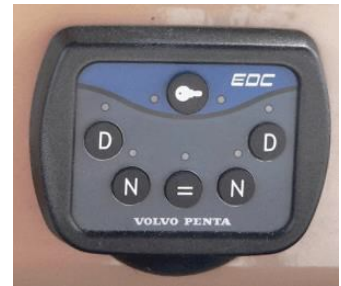
Engine control “Key” and “N” buttons
