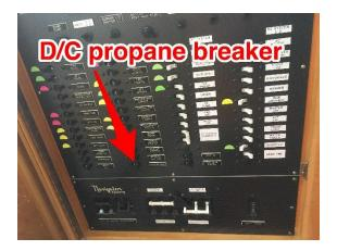
Turn the A/C Stovetop breaker to the ON position. Note: The A/C breaker controls the electronic ignition of the stovetop. The stovetop can still be used without the inverter on but it must be lit using a lighter.
