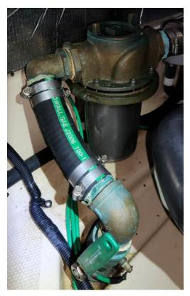
Observe the glass of the RAW WATER <u>S</u>TRAINER for debris. If necessary, <u>close the sea cock</u>, open the strainer cover, clean the strainer, and reassemble. **Remember to reopen the sea cock**.
