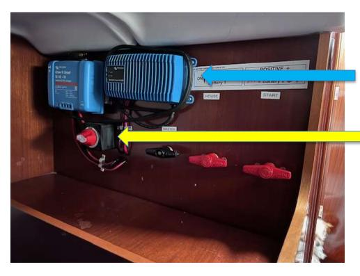
110V House battery charger can be plugged into shore power (110V outlet).
