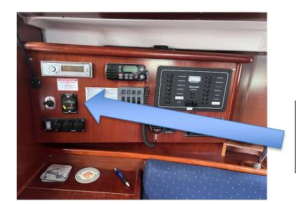
Windlass Breaker pictured in the normally open–off position. Push yellow lever up until it clicks to closed-on position.
