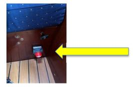
House Solar Switch pictured in the off position. For duration of your cruise, Turn 90 degrees to vertical to connect the lithium battery to solar panels for recharging. If solar charging is insufficient to maintain the house battery charge day to day, the house battery can also be charged via the engine's alternator by turning the DC to DC switch to vertical. Never turn switches while the engine is operating as electrical system damage may occur.
