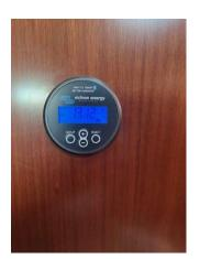
Alternatively, the house battery can be monitored directly via a free phone app called My-BMS that connects directly to the lithium battery via bluetooth. Select the "12V-300Ah" device. Then select the control panel.
