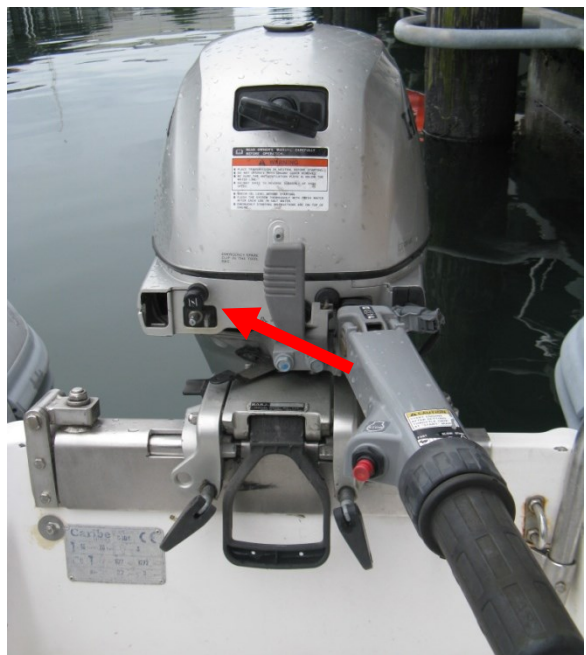
OUTBOARD MOTOR SHOWING GAS CONNECTION AND CHOKE
