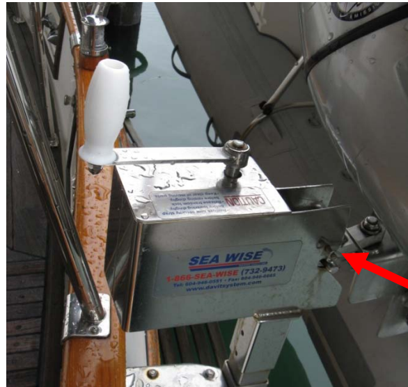
DAVIT CRANK AND SAFETY PIN
