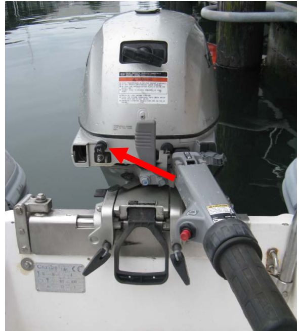
OUTBOARD MOTOR SHOWING GAS CONNECTION AND CHOKE LEVER
