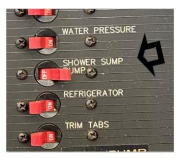
NOTE – If SUMP PUMP stays ON, debris may have built up on the sensor switch. Open the box lid, lift out the cylinder-shaped strainer. Wipe scum from switch and pump. Replace strainer and lid.
