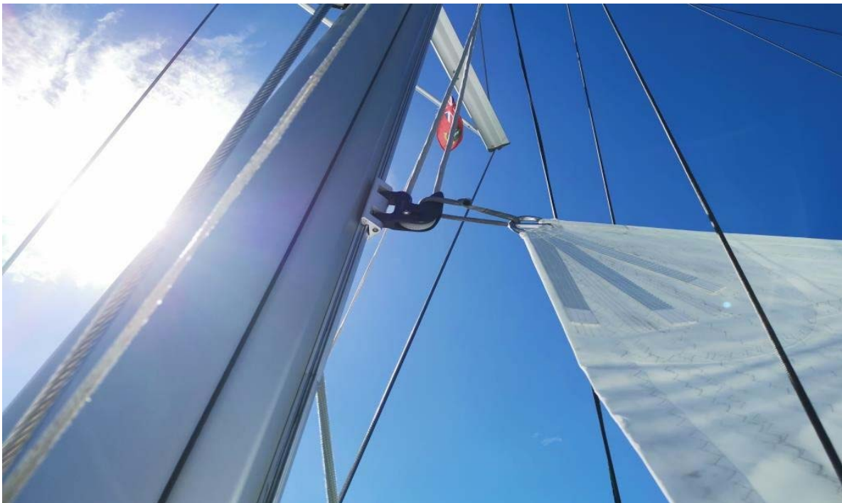
Pic 3. Looped line sitting on Halyard hook.
