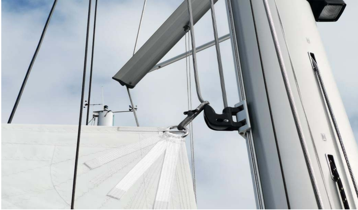
Pic 4. Loop not engaging hook.
