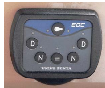
Engine control “Key” and “N” buttons
