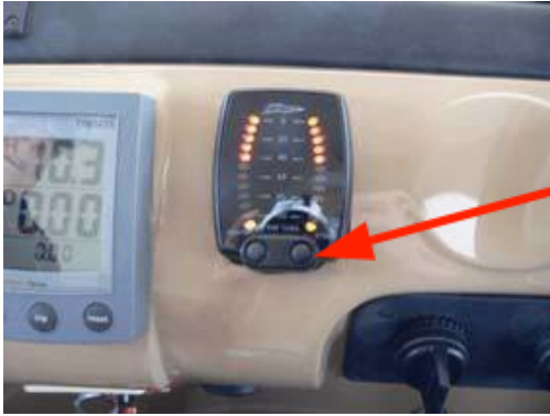
Trim tab indicator, tabs half down.
