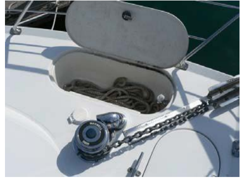
Looking at the anchor windlass and chain. Just above the windlass with the white cover is one of the footswitches; at the top is seen one of the two deck hatches to hold anchor bridle, dock lines, etc. Washdown faucets are here as well.
