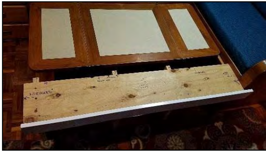
10. Stand supporter upright; lift table enough to slide supporter underneath.
