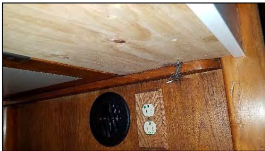
11. Attach hook under aft end of supporter to settee frame.
