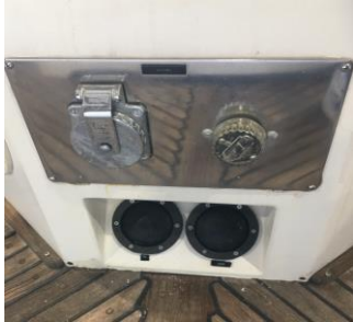
Forward power connection
