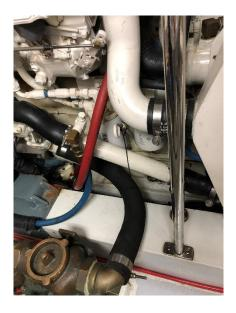
Ensure the valve on each RAW WATER THRU-HULL, located on the port side of the engine is in the 'open' position (lever in-line with valve). Observe the glass of each RAW WATER STRAINER for debris. If necessary, close the seacock, open the strainer cover, clean the strainer, and reassemble. Remember to reopen the seacock. Check your generator fluids as well. Confirm water flow in exhaust after reassembling strainer and starting engine.
