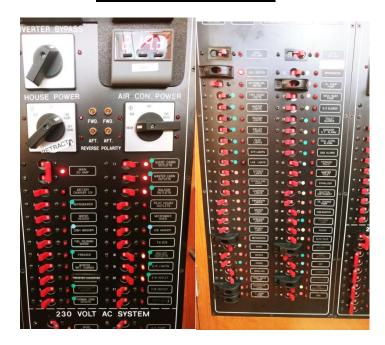
The electrical system is divided into two distribution systems: 120-volt AC and 12-volt DC.
