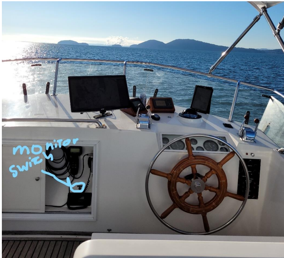
Flybridge, note location of radio, autopilot and toggle switch for monitor.
