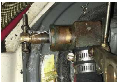
Figure 2 - Seacock for raw water
