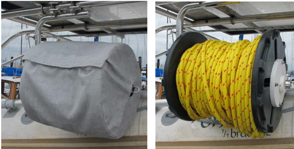
Figure 12: Stern Tie Reel, covered and uncovered
