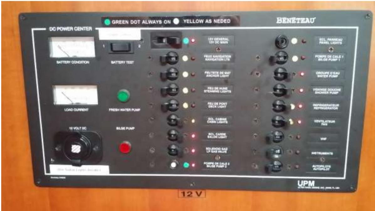
The 12-volt DC panel shows all the systems supported by your batteries. Primarily you will be turning on the breakers for your lights, water pressure, electronics, etc. Interior lights are also powered from a circuit breaker on this panel but many have individual switches at each fixture. #2 Bilge pump light is always on. Breakers such as the LP gas breaker should always be turned off after every use.
