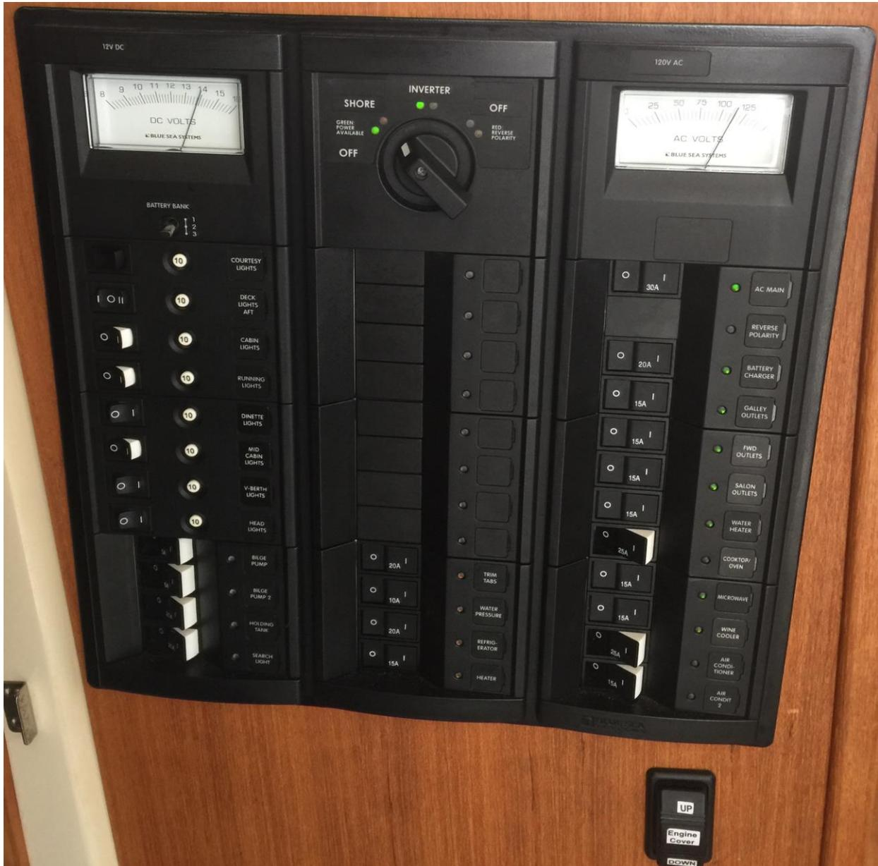
SHORE POWER supports all AC equipment and receptacles on board, as well as the battery charger. Before connecting to shore power, ensure the circuit breaker switch on the ELECTRICAL PANEL labeled AC MAIN is in the off position. Also, switch all breakers on the ac panel to off to avoid a power surge when turning on the main.
